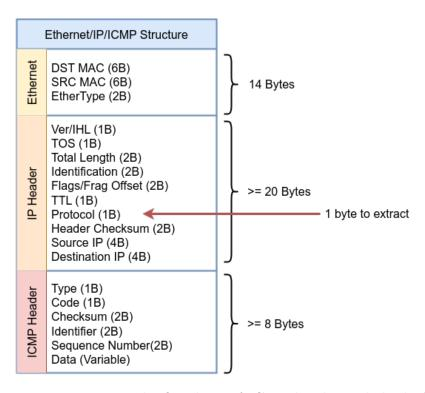
Then the last part is moving to the first byte of ICMP header and check if the packet is echo request or drop the packet from the socket. Finally, return skb->len indicated that the packet should be accepted and passed along to user space or to further processing. Let's move to the user-space code.
