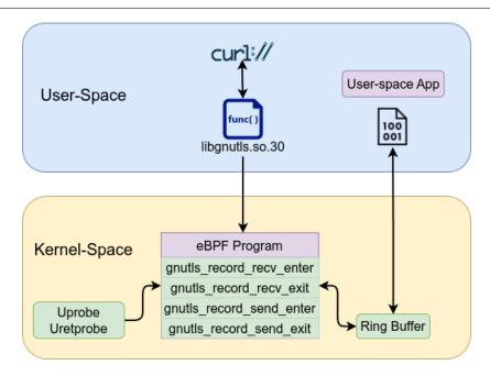
To capture the decrypted or plaintext data processed by these functions, you need to attach uprobes at both the entry and exit points of each function. Attaching a probe at the entry captures the buffer pointer as it is passed to the function, while attaching a probe at the exit allows you to read the final processed data from that buffer once the function has completed its work.
