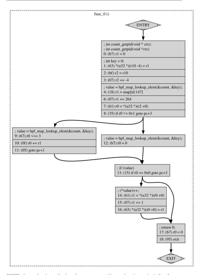
BPFTool can also dump jited or the program machine code using sudo bpftool prog
