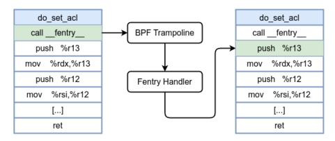
Let's see the following example, which attaches a probe to the entry of do\_set\_acl kernel function. do\_set\_acl is a kernel function that implements the setting of Access Control Lists (ACLs) on files and directories, enabling granular permission control beyond standard Unix permissions.
