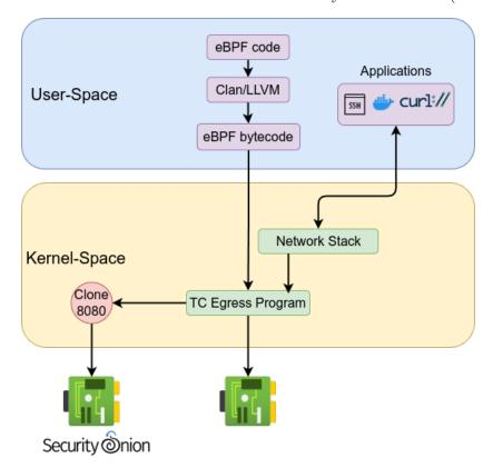
The next example demonstrates one of the capabilities of traffic control—manipulating traffic. In this example, the program will change the first 4 bytes of an HTTP response (initiated from port 8080) to 'XXXX'. This means that instead of seeing 'HTTP/1.0', you would see 'XXXX/1.0'.
