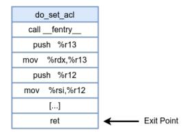
After inserting an fexit probe (with BPF trampoline):
