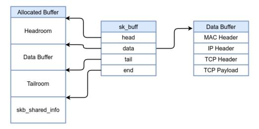
\_\_sk\_buff data structure is a simplified version of sk\_buff structure that's exposed to eBPF programs. It provides a subset of information about a network packet that eBPF programs can use to inspect, filter, or even modify packets without needing access to all the internals of the full sk\_buff.
