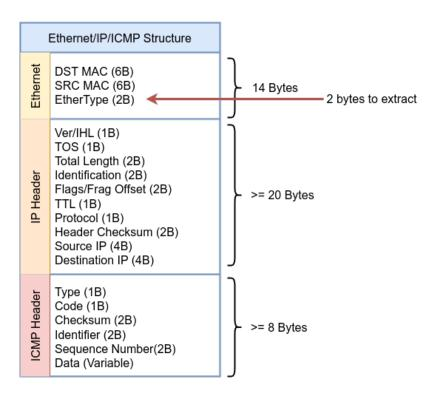
bpf\_skb\_load\_bytes helper function will do that bpf\_skb\_load\_bytes(skb, ETH\_TYPE, &eth\_proto, sizeof(eth\_proto)), it will extract EtherType for us and save the output in eth\_proto. We define eth\_proto as \_\_u16 which is unsigned 16-bit integer and that's why bpf\_skb\_load\_bytes will extract in that case 2 bytes because we specified the length we need as sizeof(eth\_proto).
