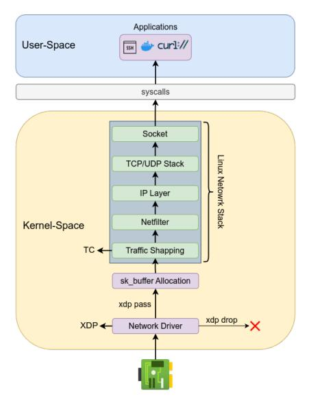
One common use case of XDP is DDoS mitigation, where it quickly identifies and drops malicious traffic with minimal processing overhead. XDP is also heavily used for advanced packet forwarding and load balancing, enabling quick header modifications and packet routing decisions directly at the driver level.
