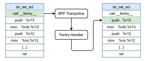
Let's explore the following example which is attach a probe to return of do\_set\_acl kernel function.
